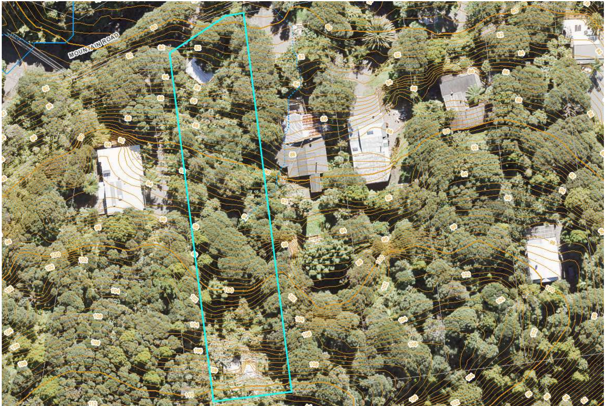
Figure 1. Aerial view of the site outlined in light blue, with contours. The existing garage is visible in the top of the photo and the ruins of the previous dwelling in the bottom. The road visible in the top left is Mountain Road. Image Auckland GeoMaps.
